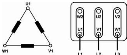
Delta connection is obtained by connecting the end of a phase to the beginning of the next phase.
