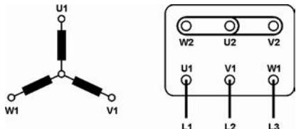
Star connection is obtained by connecting terminals W2, U2, V2 to each other and terminals U1, V1, W1 to the mains.
