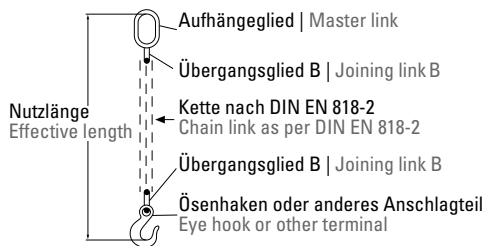
Form H 1 Hakenkette 1-strängig Single leg sling with hook
